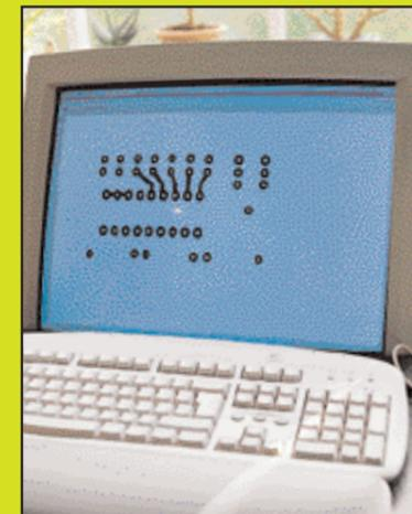
1 I use a simple PC drawing package to draw the circles where I'm going to drill holes in the board for the component's legs. Spacing is based on a 0.1 inch grid. The tracks are 1mm wide, the circles 2mm diameter and the holes 1mm. ◀ ▶
