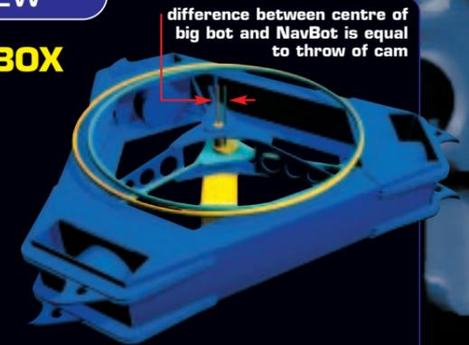
together on a 'live' axle. This resists the torque [turning force] applied by the steering cam linkage [the wobble box]. In line with this live axle is a gearbox and a motor – which is also free to turn with the wheels."
