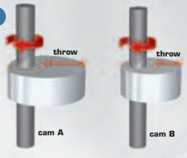
second tops, and the key things that make them do this are the speed of rotation (1000rpm), and the amount by which each wheel steers out and in per rev (3°). That 3° is pinned down by the amount of 'throw' the cam has (0.25 inch) (see Need to Know). But why not give it more throw and make the robot faster?
